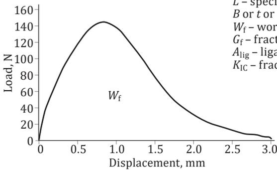
**Figure 5.** Test setup and typical Load-Displacement curve (a) SCB (b) SENB (Abu Abdo et al., 2014)
