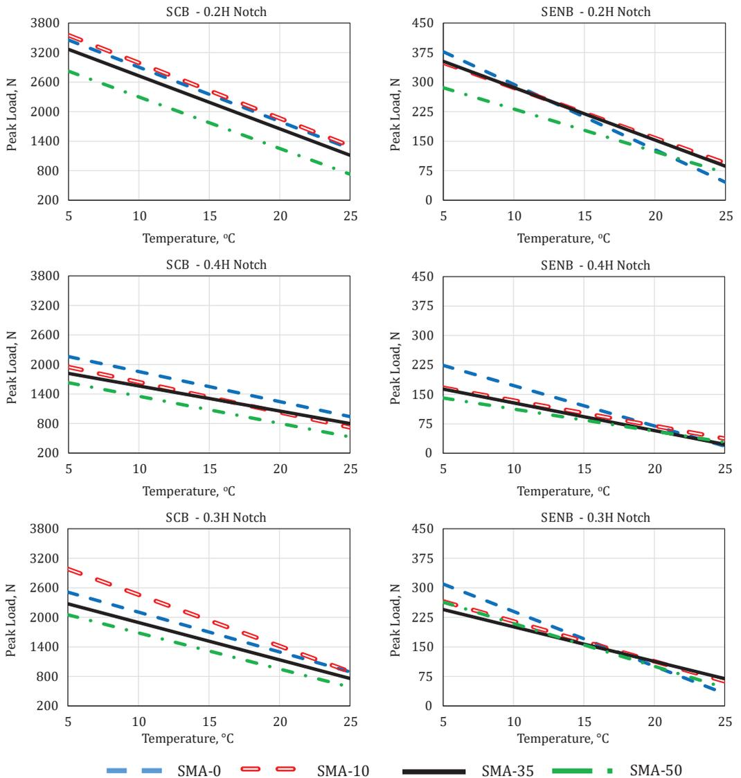
**Figure 10.** Peak load vs. temperature for varying notch depths
