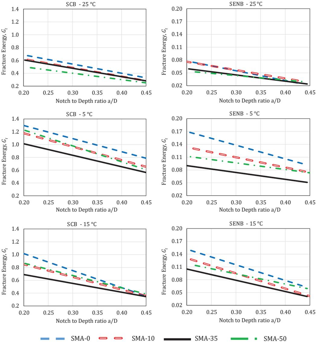
Figure 11. Fracture energy vs. notch depths for varying temperatures
