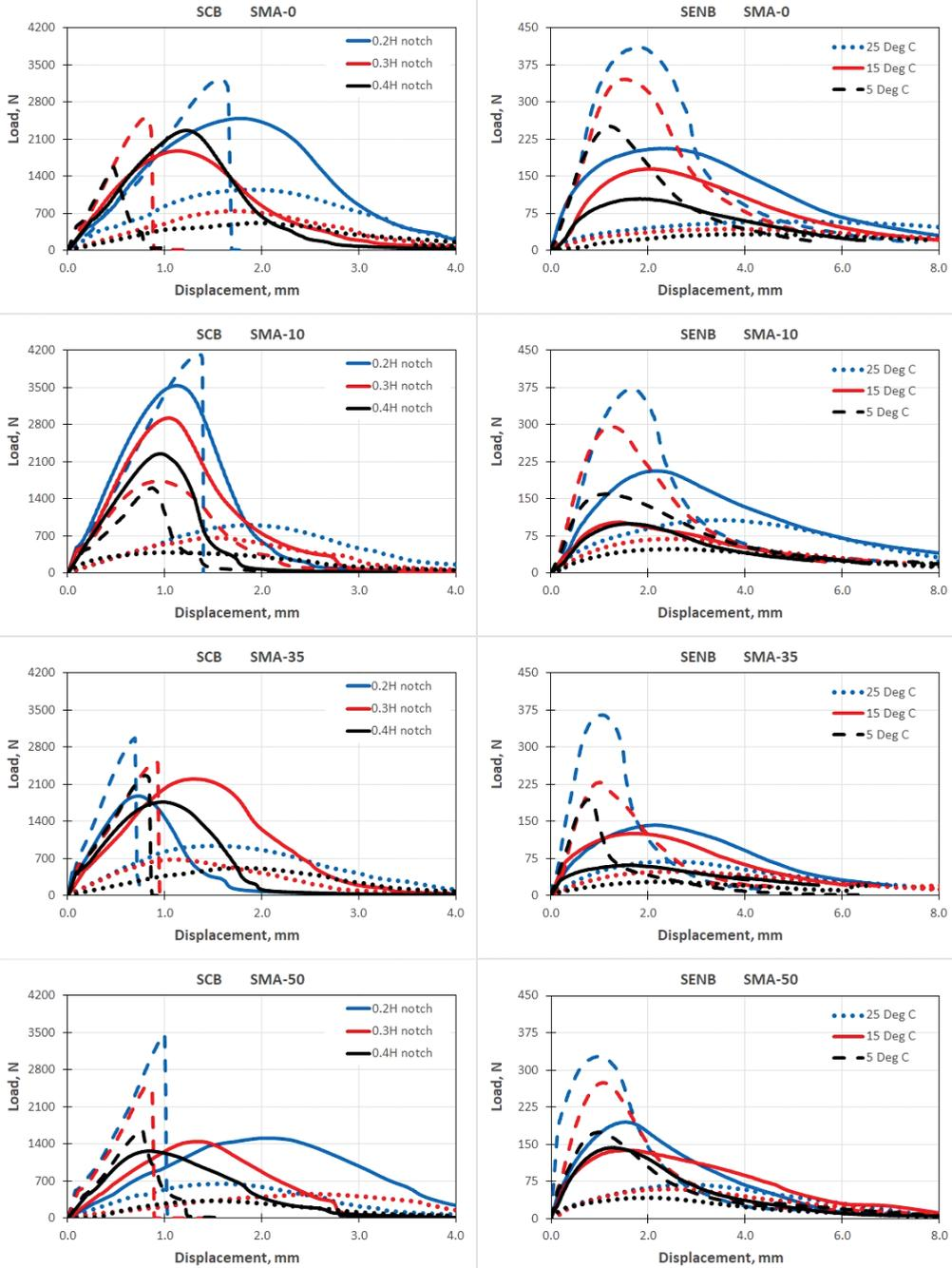
**Figure 8.** Load–displacement curves of SCB and SENB tests at varying notch depths and temperatures
