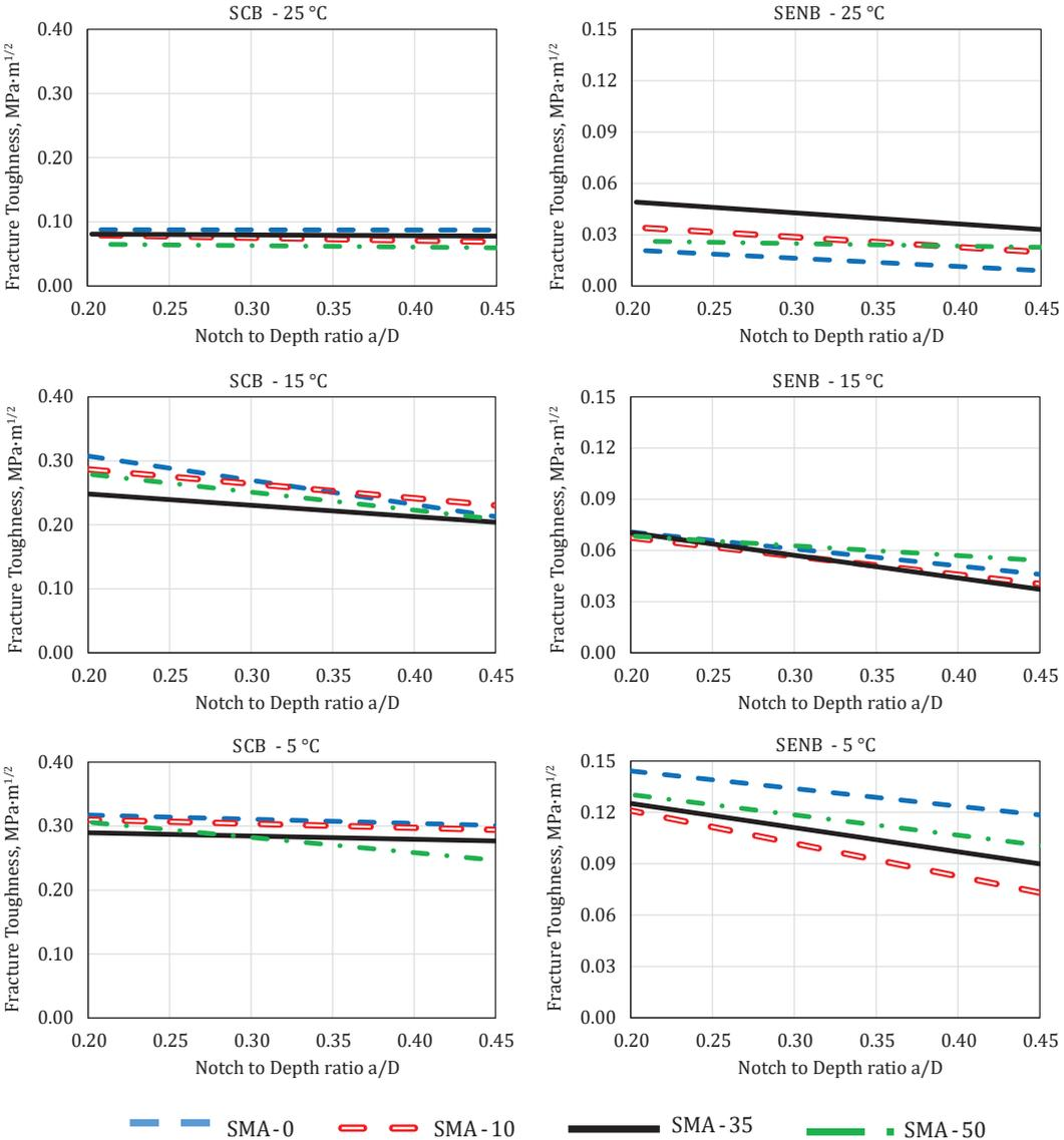
**Figure 13.** Fracture toughness vs. notch depths (a) 25 °C; (b) 15 °C; (c) 5 °C
