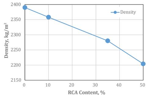
**Figure 6.** RCA-SMA properties (a) stability and flow; (b) VMA and VFA; (c) ITSM and OBC; (d) density
