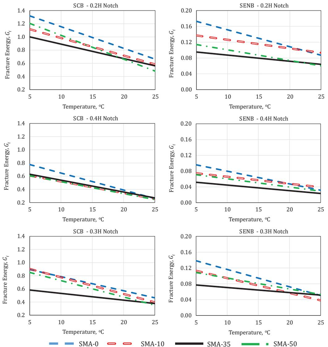
Figure 12. Fracture energy vs. temperature for varying notch depths
