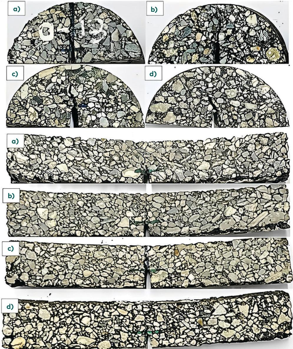
**Figure 7.** Cracks in SCB and SENB samples (a) SMA-0; (b) SMA-10; (c) SMA-35; (d) SMA-50
