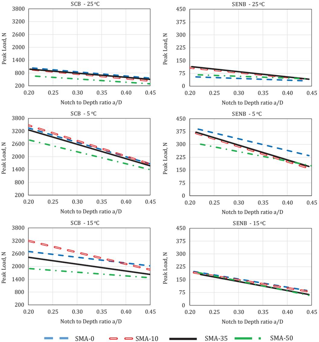
Figure 9. Peak load vs. notch depths at varying temperatures
