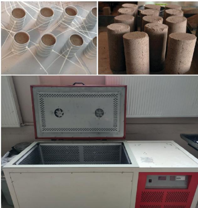
**Figure 3.** Prepared samples and freezing-thawing machine
