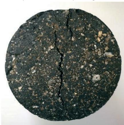
(b) A specimen after freeze-thaw splitting test
