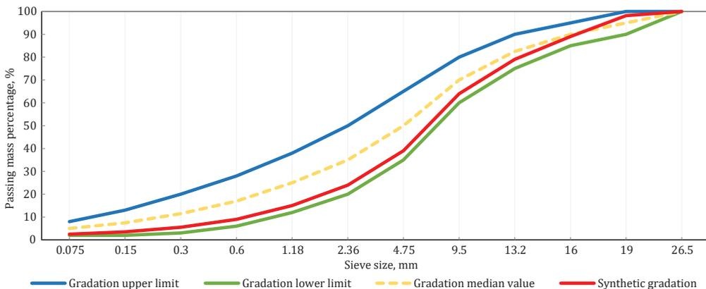
Figure 1. Gradation curve of EACRM
