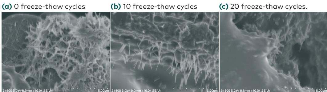
**Figure 9.** Micro-morphology of the cement emulsified asphalt mortar of the cold recycled mixture under different freeze-thaw cycles
