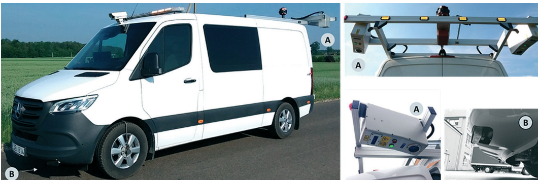
Figure 1. Mobile road research equipment RST63 (A – LCMS-2 lasers; B – point type lasers)
