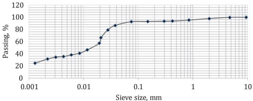
Figure 4. Grain size distribution curve of expansive soil
