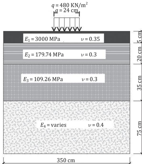
**Figure 3.** Wheel Load applied on pavement and section properties
