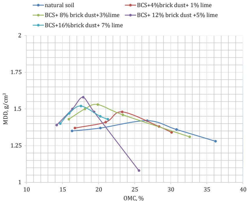
**Figure 6.** Effects of brick dust-lime on dry density-moisture content of expansive soil
