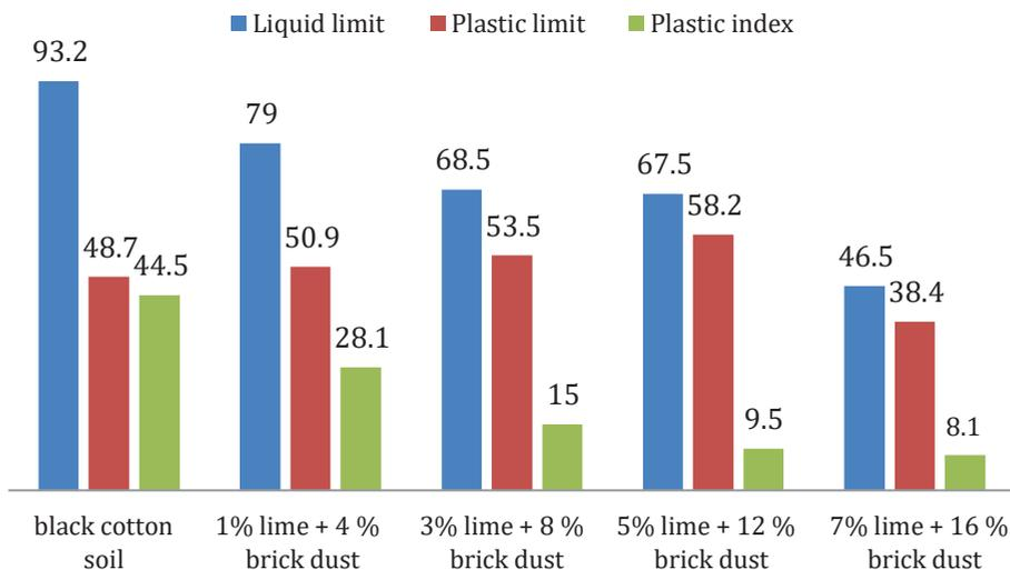
**Figure 5.** Effect of brick dust-lime on Atterberg limit results
