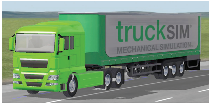
Figure 3. A 3-axle cab with a 3-axle European trailer
