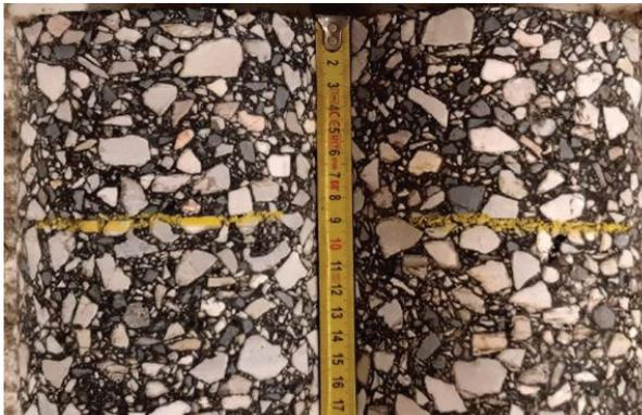
**Figure 2.** AC22 binder (F) B70/100 (50%RA) – on the top – and AC22 binder (F) B70/100 (40%RA) – bottom
