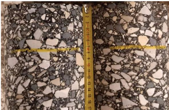
**Figure 3.** AC22 binder (F) B70/100 (60%RA) – on the top – and AC22 binder (F) B70/100 (40%RA) – bottom
