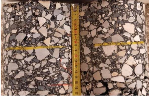
**Figure 1.** AC22 binder (F) B70/100 (50%RA) – on the top – and AC22 binder (F) B70/100 (30%RA) – bottom
