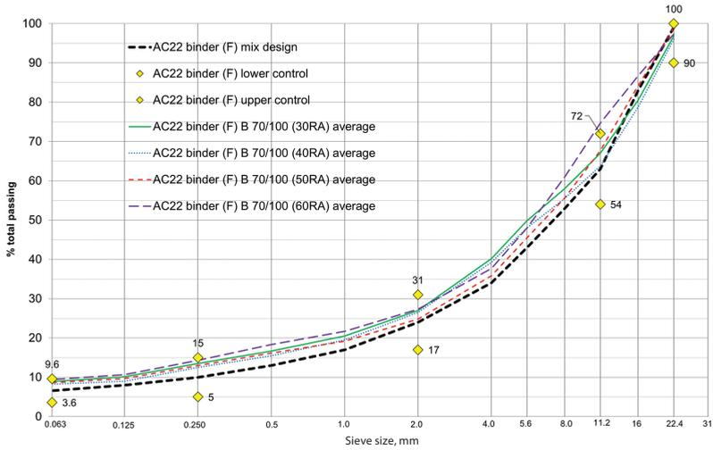
**Figure 4.** Particle size distribution of AC22 binder (F) asphalt mix manufactured with plain binder and various RAP contents, plant mixed asphalt
