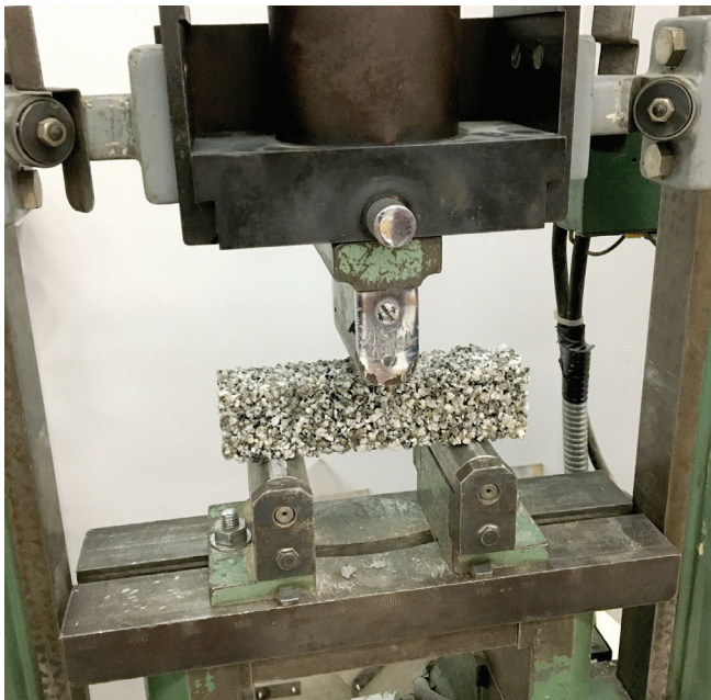
Figure 4. Flexural test of sample made with aggregate no. 1
