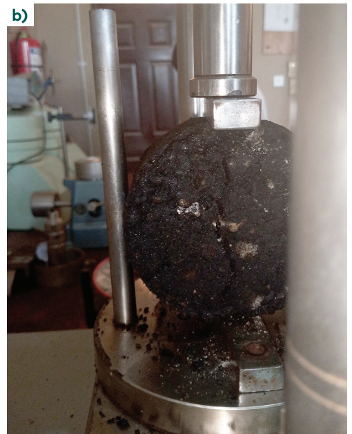
Figure 4. Specimen under Indirect Tensile Strength test (a) and (b)
