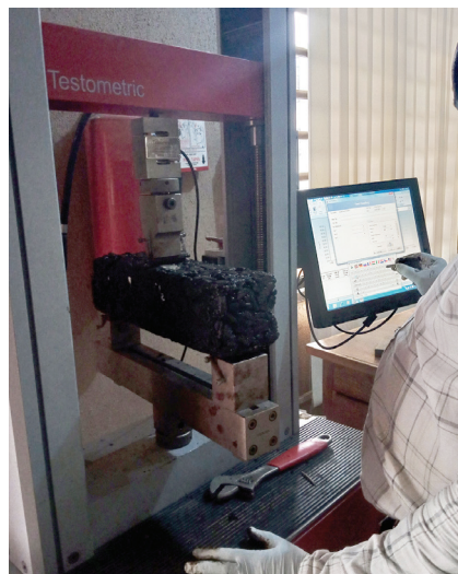
Figure 2. Beams test setup for three-point load
