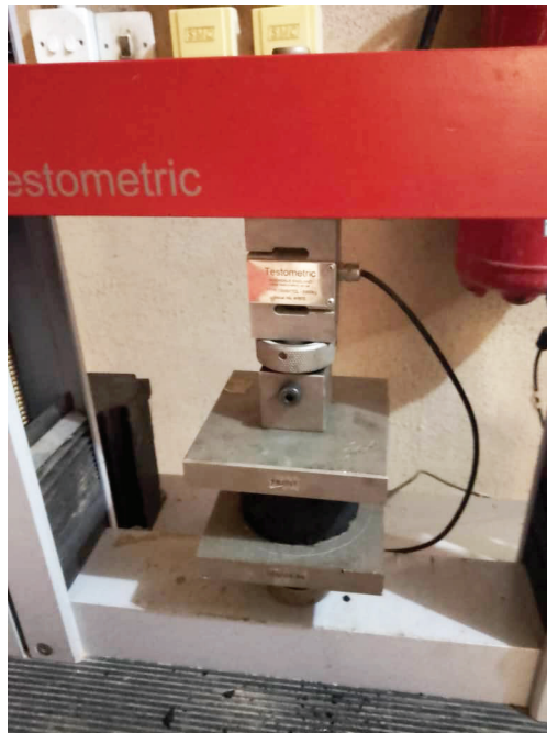
Figure 5. Specimen under Universal Testing Machine for compression test
