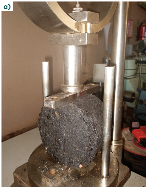
Figure 4. Specimen under Indirect Tensile Strength test (a) and (b)
