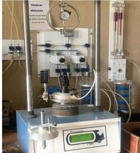
Figure 3. Specimen failure in the triaxial testing machine
