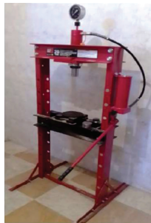
Figure 3. UCS hydraulic press and extruder of samples
