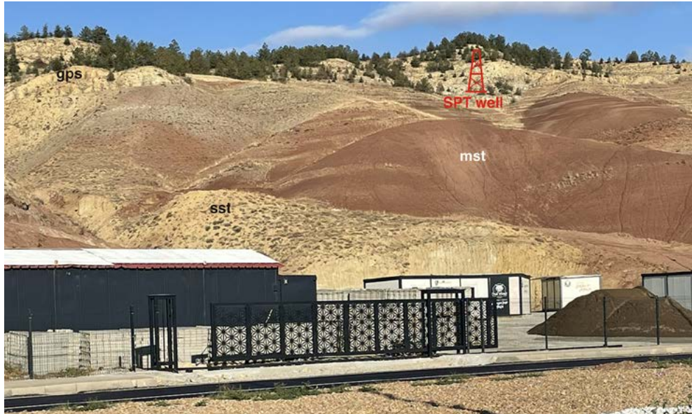
Figure 7. The SPT used in the area located in the dark brown-reddish mudstones (mst) and thin-grain sandstones (sst) containing gypsum (gps) layers
