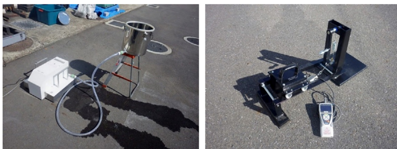
Figure 12. Photographs of the DFT and ONO-PPSM device
