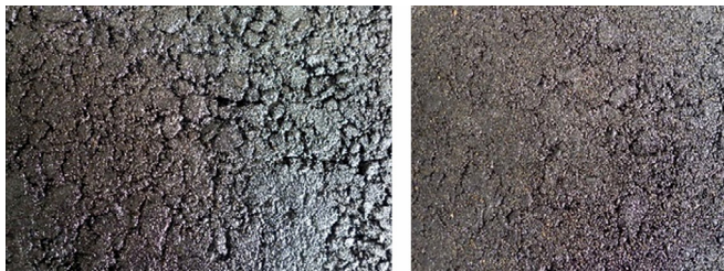
Figure 7. Surfaces of dense-graded and fine-graded asphalt mixtures
