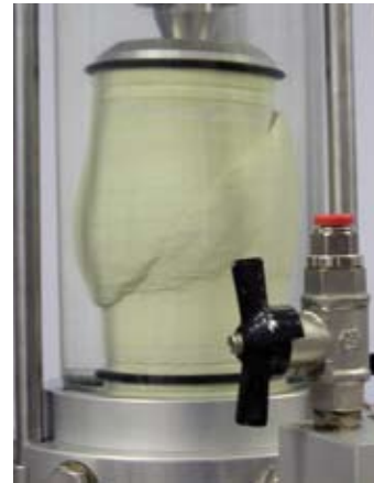
Fig. 8. Triaxial test dense sand sample of H/D = 2
