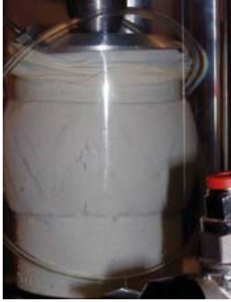
Fig. 11. Triaxial test dense sand sample of H/D = 1
