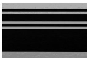
Fig. 3. Scale fragment of a coded leveling staff
