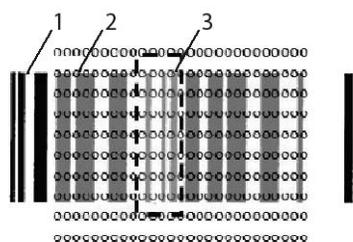
Fig. 2. Principal system of calibration: 1 – coded bars of the staff; 2 – array of CCD sensors; 3 – analyzing window
