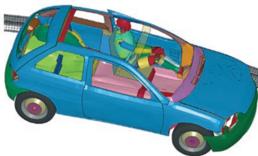
Fig. 7. Safety barrier simulation with rigidly belted Hybrid III dummy
