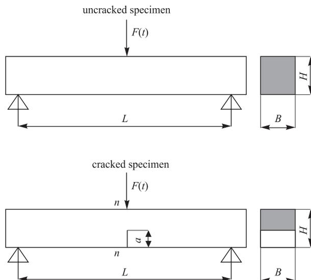
Fig. 1. Specimen's types, where  $L$  – length;  $B$  – width;  $H$  – height,  $a$  – crack length
