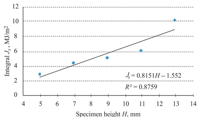
**Fig. 3.** Relationship between  $J_S$ -integral and specimen's height  $H$
