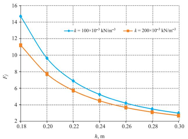
**Fig. 3.** Equivalent axle load factors  $F_j$  obtained from Portland Cement Association criterion in relation to thickness of concrete slab  $h$  and modulus of subgrade reaction  $k$  (for standard axle load  $Q_s = 100$  kN and actual axle load  $Q_j = 120$  kN)
