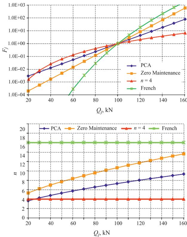
**Fig. 1.** Equivalent axle load factors  $F_j$  and exponents  $n$  in relation  $F_j = \left(\frac{Q_j}{Q_s}\right)^n$  obtained from various fatigue criteria as a function of actual axle load  $Q_j$  (for  $h = 0.26$  m,  $R_b = 5.5 \times 10^3$  kN/m<sup>2</sup>,  $E = 35 \times 10^6$  kN/m<sup>2</sup>;  $k = 100 \times 10^3$  kN/m<sup>3</sup>,  $Q_s = 100$  kN)
