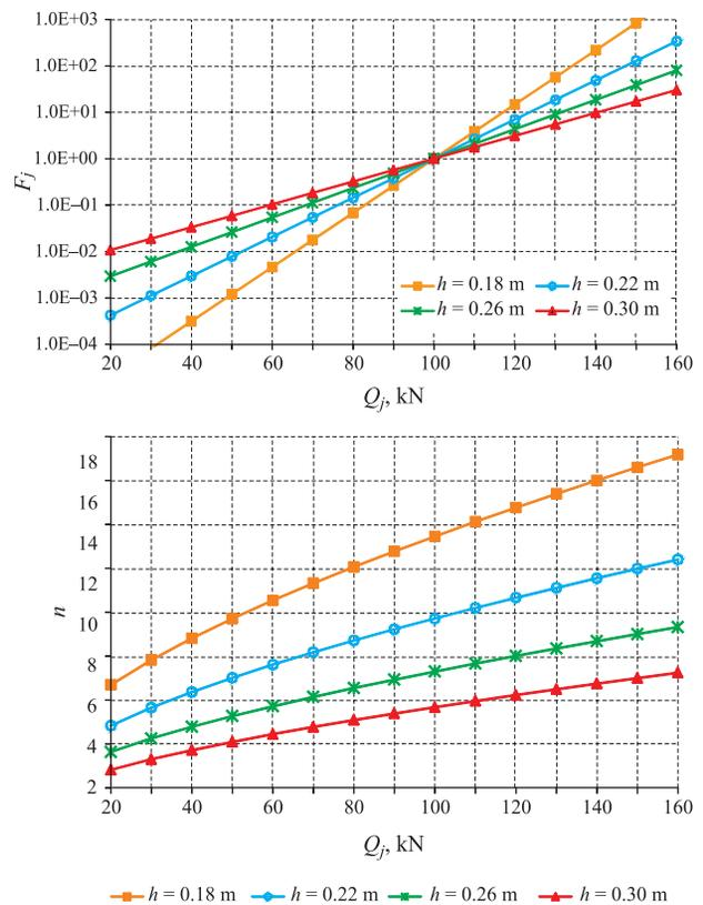
**Fig. 2.** Equivalent axle load factors  $F_j$  and exponent  $n$  in relation  $F_j = \left(\frac{Q_j}{Q_s}\right)^n$  obtained from Portland Cement Association criterion as a function of actual axle load  $Q_j$  and thickness of concrete slab  $h$  (for  $R_b = 5.5 \times 10^3$  kN/m<sup>2</sup>,  $E = 35 \times 10^6$  kN/m<sup>2</sup>;  $k = 100 \times 10^3$  kN/m<sup>3</sup>,  $Q_s = 100$  kN)
