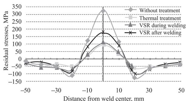
Fig. 2. Distribution of longitudinal residual stresses in specimens by ultrasonic technique
