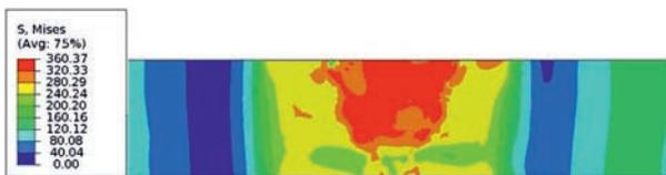
Fig. 4. Distribution of von Mises stresses, MPa
