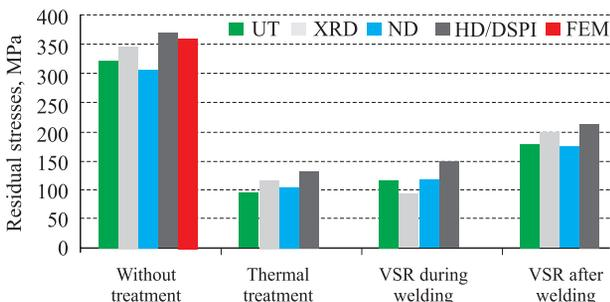
Fig. 5. Peak of longitudinal residual stresses in welded specimens, using different measurement techniques
