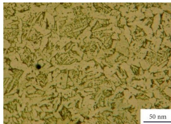
Fig. 9. Microstructure of welded metal (VSR during welding)
