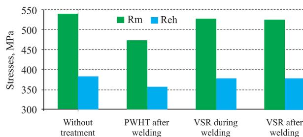
Fig. 6. The tensile test results
