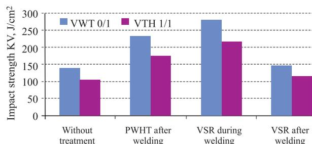
Fig. 7. The impact strength test results
