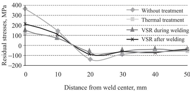
Fig. 3. Distribution of longitudinal residual stresses in specimens
