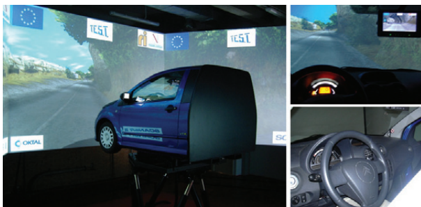
Fig. 1. The VERA driving simulator
