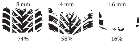
Figure 4. Dependence of the contact zone on the tread height
